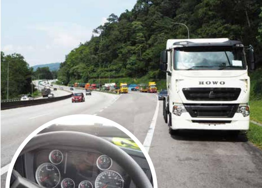
density 50 percent less and higher stability. With this, the brand can guarantee one million kilometres without deformation. The T7H can be configured to be in 4X2/6X2/6X4 drive trains and engines ranging from Euro III: 350/390/430/480/540.
