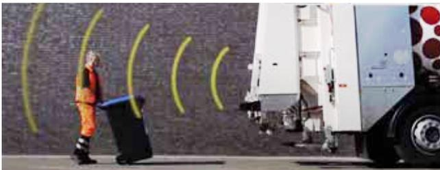
Automously brakes the reversing trailer at a programmable distance from detected objects. Actively warns the driver by pulsing the brakes when the reversing speed is higher than 9km/h
