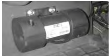
Fatigue vibration motor installed at the back of the driver's seat
