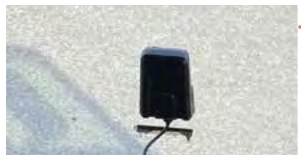
Front alert camera installed at the center of the wind screen facing the road
