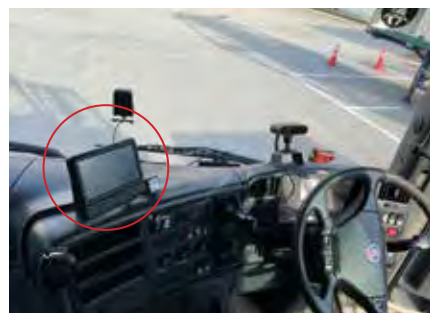
LCD monitor screen installed on dashboard
