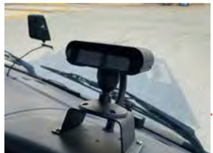
Driver alert system installed on dashboard facing the Driver
