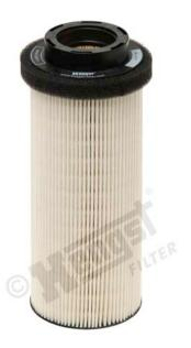
Original Hengst Filter E82KP suitable for DAF, RENAULT. Top/bottom end plastic discs are heated up to insert the filter media into the plastic to ensure a perfect seal.
