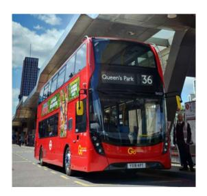
lexander Dennis Limited (ADL) and BAE Systems have delivered the first 39 Enviro400H double-deck buses with Series-E hybrid technology to launch customer Go-Ahead London. Using ultra-capacitor energy storage to further reduce life cycle costs, this
