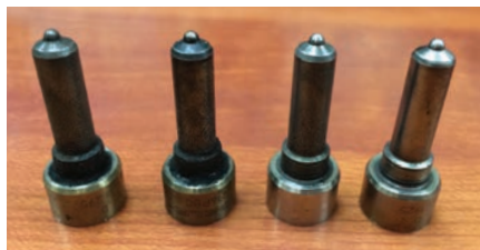
Unlike the rest, the injector on the far right used only Shell FuelSave Diesel and stayed clean from deposits.
