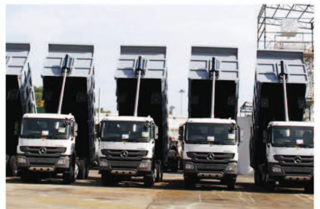
Hydraulic Tipping Hoists
