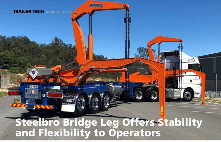
teelbro is expanding its product options in Malaysia with the Bridge Leg. The Bridge Leg is an optional crane/leg for Steelbro SB362 36 Tonne lifting capacity Sidelifter. It offers customers an alternative to the standard tilt and extend stabiliser legs and provides flexibility for all operations.
