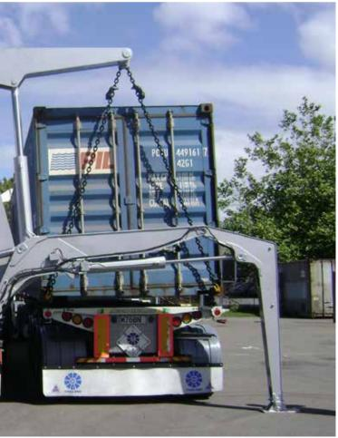
spaces or when it is difficult to align the vehicles. For an even more sturdy lifting position, the bridge leg can be fully deployed. When the Leg is deployed in the kneeling position two sensors identify the presence of a companion vehicle – thus avoiding the possibility of heavy loads being lifted when the companion vehicle is not ready.
