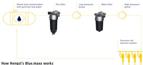
Fuel filters are indispensable for protecting the injection system and engine against contamination. This is because the requirements on diesel filtration are continuing to increase. Water and even minute particles should be effectively and reliably removed, despite very different fuel qualities. The Blue maxx fuel prefilter from Hengst is the smart solution. T
