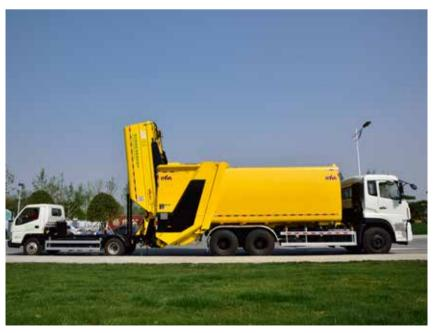
The Hyva pure electric small waste collection vehicle is an important part of Hyva's Satellite solution. The collection vehicle can match with large RCBs, and also with Hyva portable compactors, Or, it can work independently. The satellite solution is very efficient and flexible; no leakage, no pollution.
