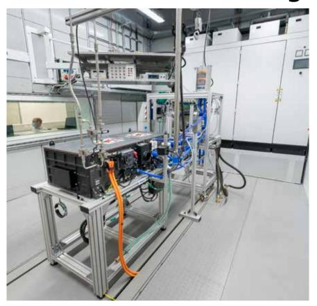
AHLE has put a new test center for hydrogen applications into operation on a 1,400-square-metre site in Stuttgart, Germany. The company has invested around EUR 2 million in the new facility, further expansion being planned. The rigs will be used to test components for fuel cells
