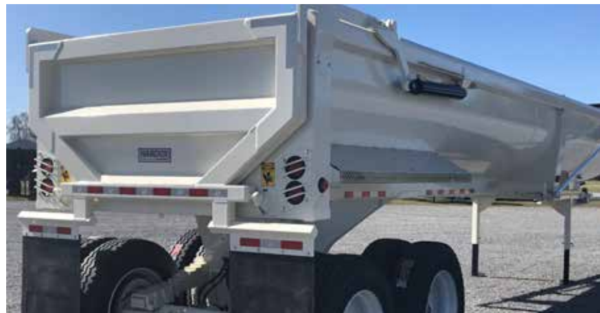
Armor Lite makes its half-round dump trailers in the new Hardox 500 Tuf wear steel.
